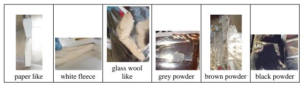
Figure 1: Different Material Groups of the Vacuum Insulation Panels
