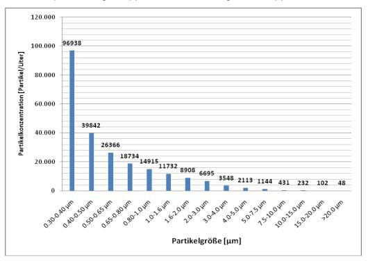
The chart below shows the averaged measurements during a time period of 2 minutes after the processing of a further 10 to 15 refrigeration appliances with VIP.
