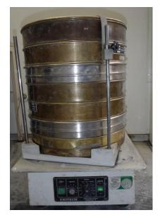
Figure 6: Sieve Tower on Mechanical Shaker
