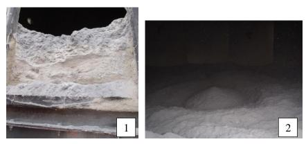
Figure 42: PU Output Mixed up with VIPs' Components (1: Layers of different Materials; 2: Interior of PU Silo)
