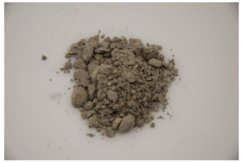
Sample 4 after 20 to 25 refrigeration appliances with VIP. Sample taken at: screw conveyor cross-flow shredder
