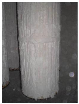
Cartridge dust filter above the cross-stream shredder after processing
