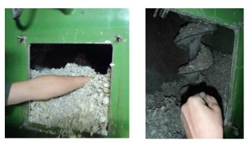
Figure 17: Opening and Cleaning of the Blocked Screw Discharge (3 Pictures)
