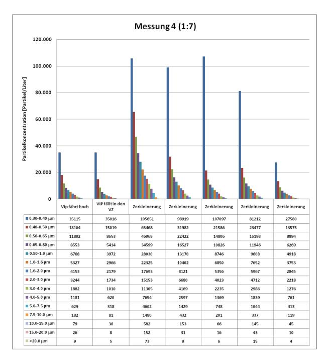
Taking into account the baseline measurement, these two charts also show that the size of the emissions and the decay curves follow similar curves. No significant increase in dust emissions can be detected between the first and last processing runs.
