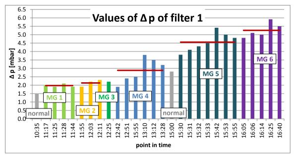
Figure 31: Measurement of Differential Pressure of Filter 1 during the Large-scale Test in TP3 (Red Lines: Average Values)
