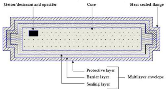
Figure 2: Schematic of a VIP from the Building Construction Industry [Alam]
