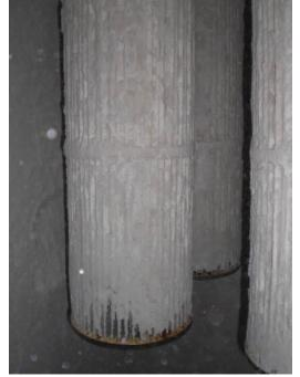
Cartridge dust filter above the cross-stream shredder before processing.
