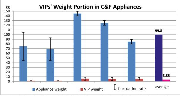
Figure 4: VIPs' Weight Portion in C&F Appliances with Fluctuation Rates (based on data from CECED)
