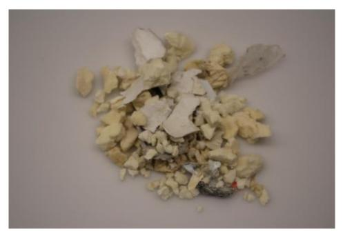
Sample 1 prior to trial. Sample taken at: screw conveyor after pre-shredder
