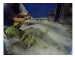
Figure 41: Residue on the Filter directly behind the Shredder
