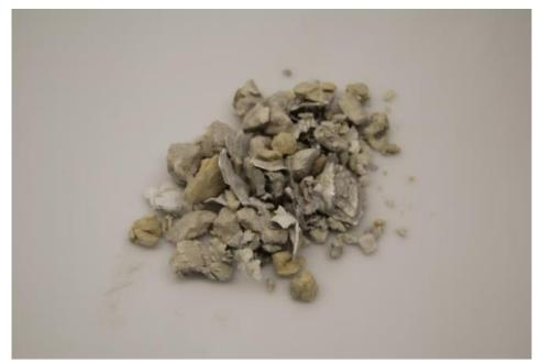
Sample 7 (combination ratio 1:5). Sample taken at: screw conveyor after pre-shredder
