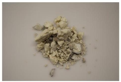
Sample 6 after 30 refrigeration appliances (combination ratio 1:7). Sample taken at: pre-shredder
