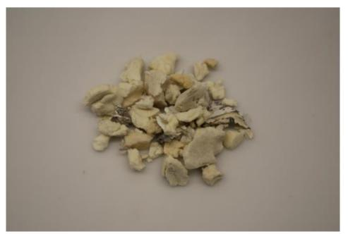
Sample 5 after 30 refrigeration appliances (combination ratio 1:10). Sample taken at: screw conveyor after pre-shredder
