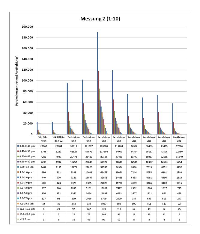
Taking into account the baseline measurement, both charts show that the size of the emissions and the decay curves follow similar curves. No significant increase in dust emissions can be detected between the first and last processing runs.
