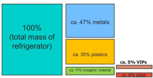
Figure 5: Mass Balance of C&F Appliances Based on an A++ Cooling Appliance [Sarc]
