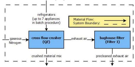
Figure 24: Schematic Diagram of the Bag House Filter (Filter 1) Directly Behind the QZ
